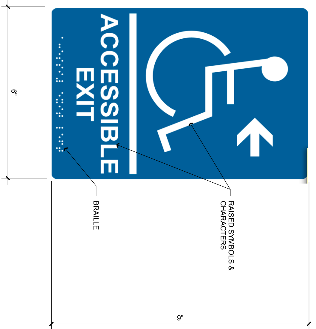
7 ACCESSIBLE EXIT SIGN SCALE: 6" = 1'-0"
