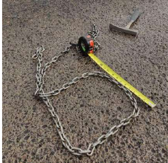
Figure 5. Chain Drag Equipment
