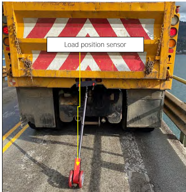
Figure 9 – Load position sensor attached to test truck (typical)
