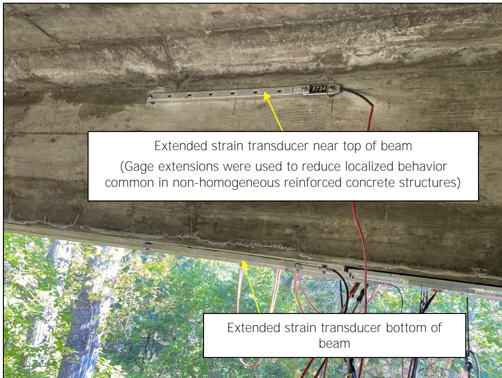
Figure 6 – Strain transducers along WA approach span concrete beams (typical)
