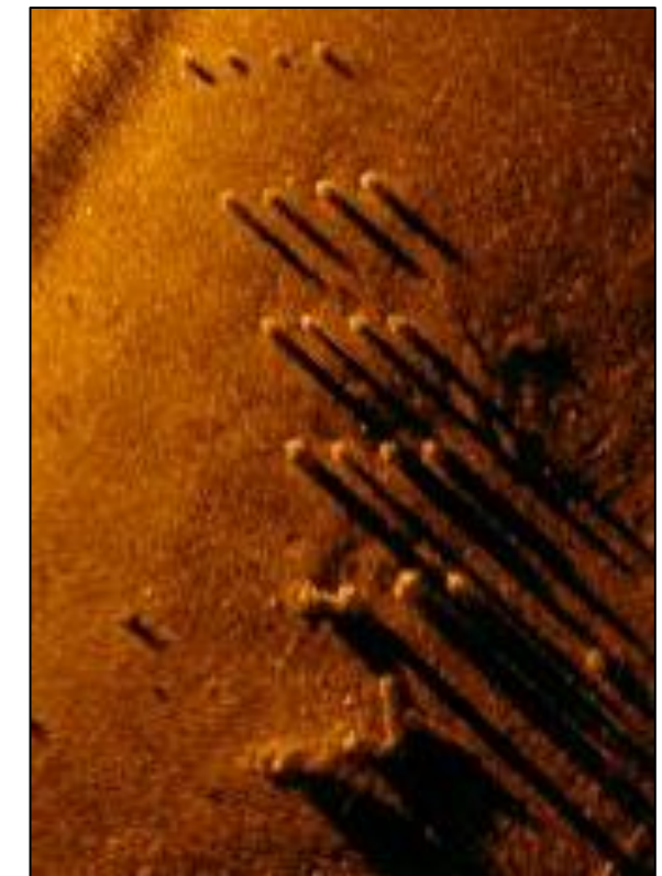
Large Piles (enlarged); note acoustic shadows.
