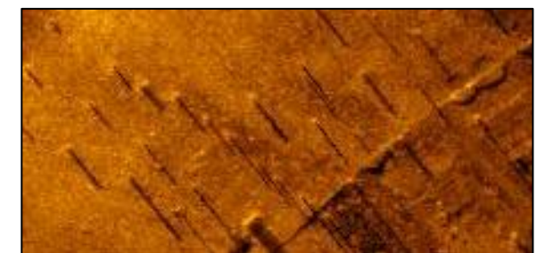
Small Piles (enlarged); note acoustic shadows.
