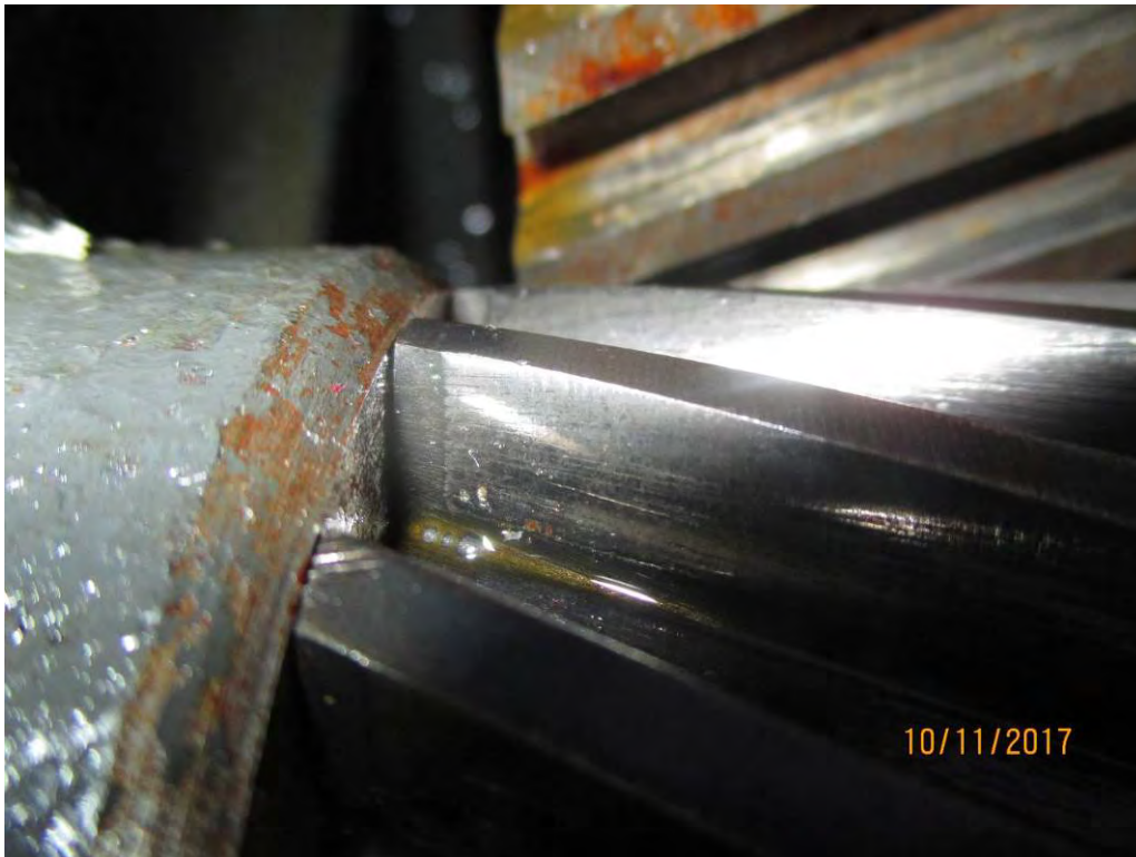
Photo 12. North Primary Reducer. View of east second reduction pinion, closing face. Small isolated pits were noted on the east (left) end of the teeth.
