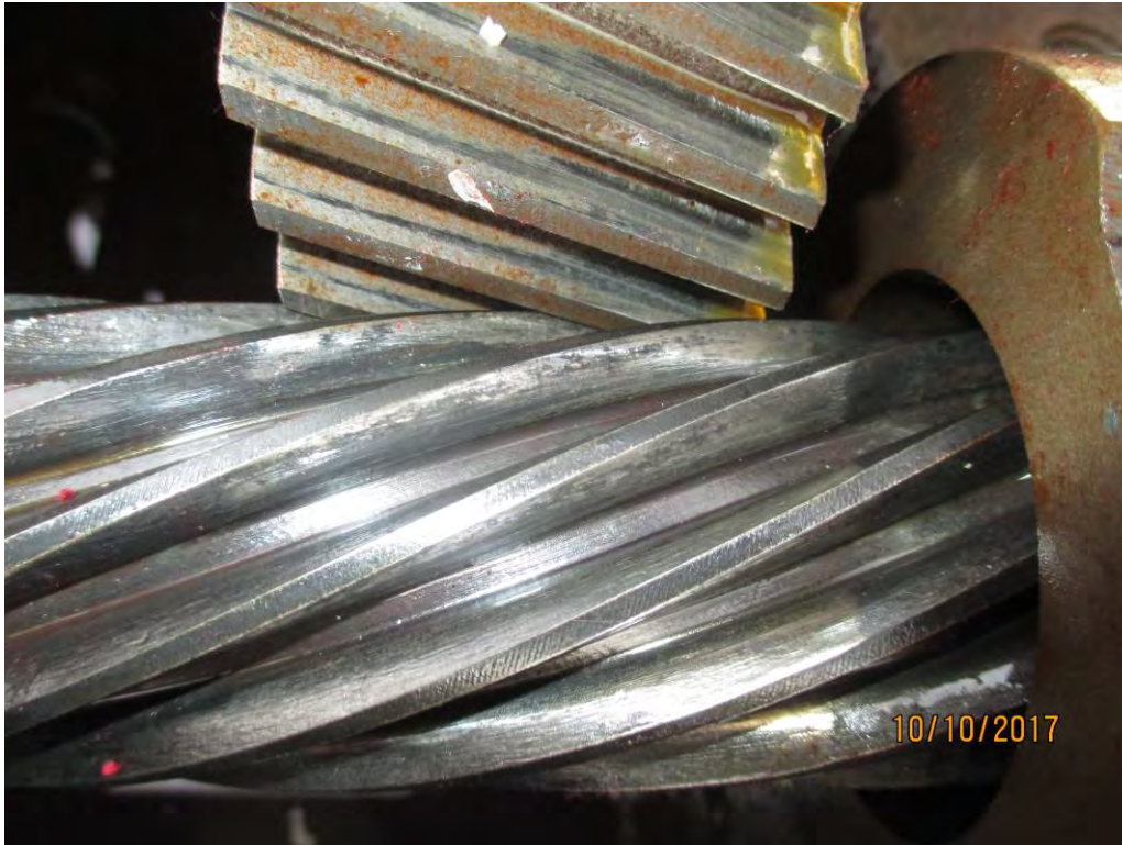
Photo 7. North Primary Reducer. View of west first reduction gear set. Note the heavier contact on the west (right) ends of the teeth.
