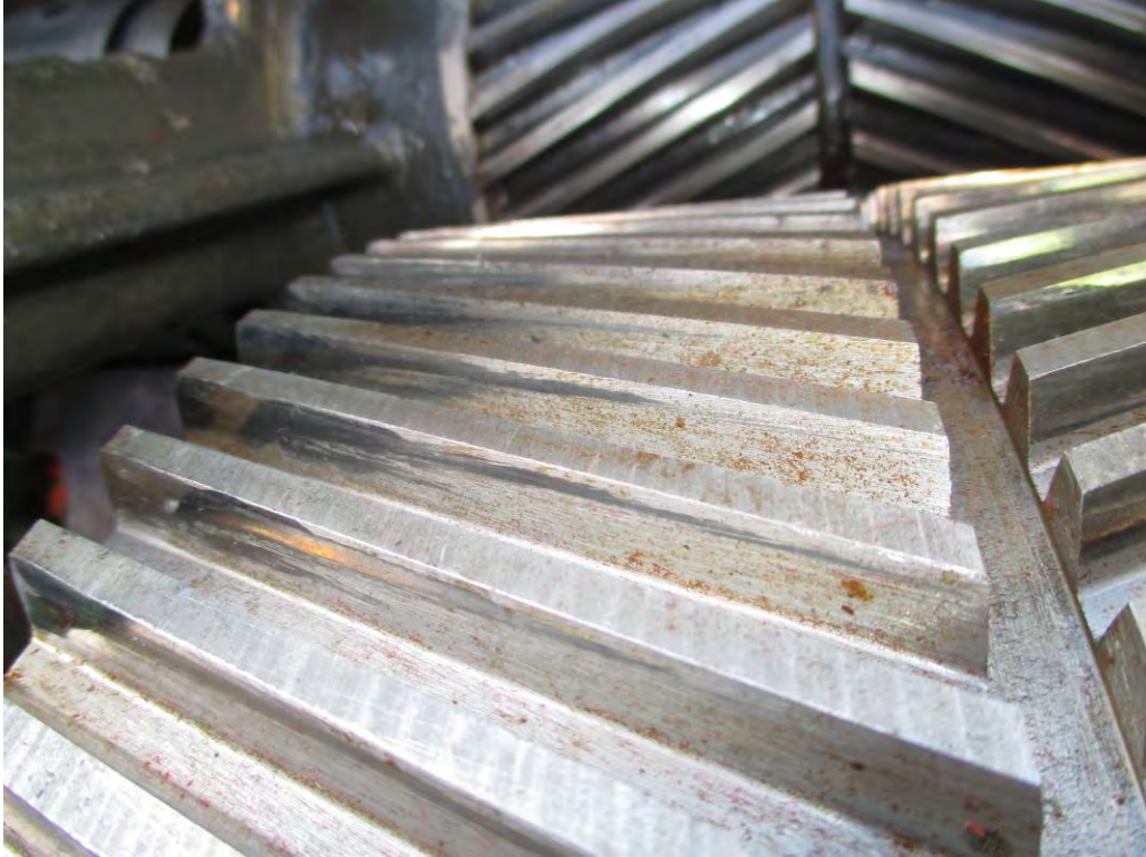
Photo 23. South Primary Reducer. View of east second reduction gear set, opening face of gear teeth. Note the contact and light wear.
