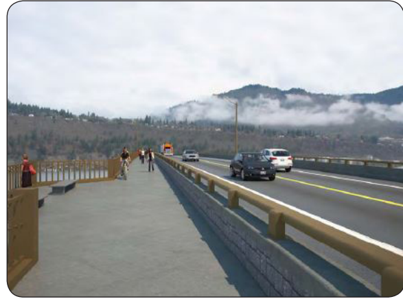
This illustration from the SR-35 Columbia River Crossing Study shows the recommended 12' wide bike/ped facility with viewpoints.
