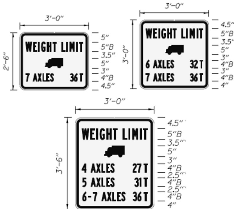
The second posting sign is to be used when both routine commercial traffic and SHVs are required to be posted for load. The following variations of the weight limit sign are designated as Sign Number OR12-5f from the ODOT Sign Policy and Guidelines, Chapter 3, page 3-111.
